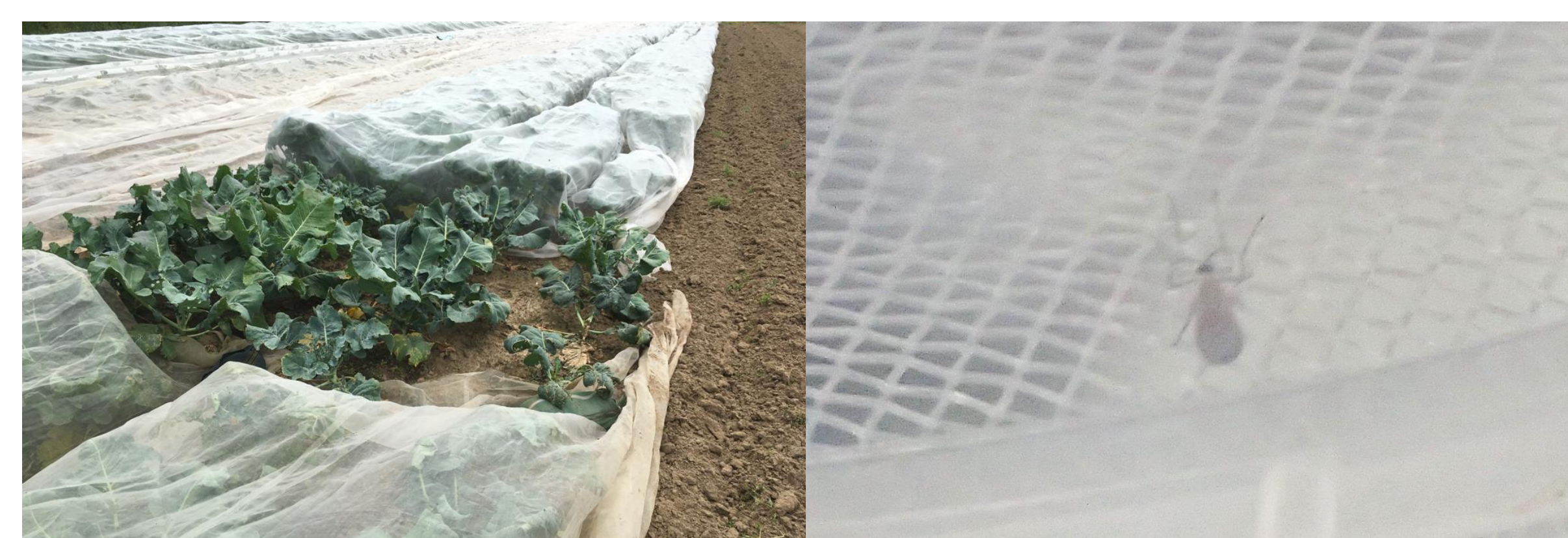
Fig. 4: Testing of the nets on-farm (left) with uncovered broccoli plants as control; and in the growth chamber (right) with an emerged midge in a small container covered with 0.6 x 0.6 mesh
